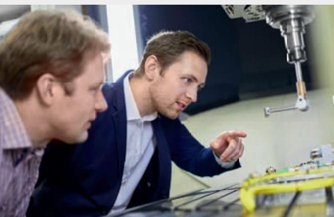
The **IDS3010** determines the effect of the combined axis deviation by measuring directly at the tool center point (from left to right: Daniel Raschke, Etalon, and Dr. Danilo Schmidt, attocube).
