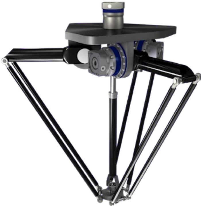
The DP+ planetary gearbox was specially developed for use in Delta robotics applications. Various characteristics allow use of the gearbox in dry, spray and wet areas (HDP+). In addition to an optimized sealing system, this drive solution includes advantages such as improved dynamics due to the optimized moment of inertia. The DP+ is available in four sizes and covers a ratio range of  $i = 16 - 55$ .
